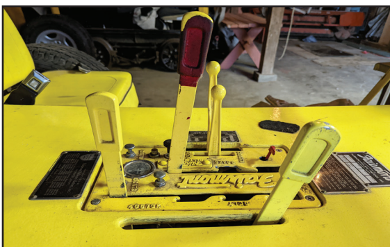
A piece of copper tubing cut in a 'V' shape was added over the starter switch to capture the lever. V bracket on right keeps the lever from going too far forward.
